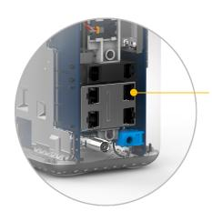
**Built for speed:** A 2.5Gbps Ethernet port to support wired speeds greater than 2 Gbps.
