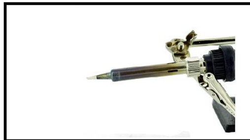
3. PROPERLY TINNED SOLDERING IRON TIP
