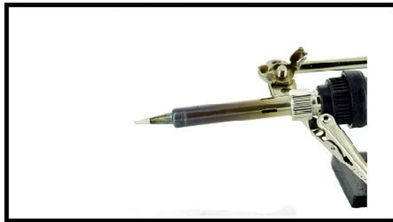
3. PROPERLY TINNED SOLDERING IRON TIP
