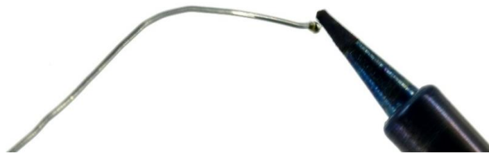
3. PROPERLY TINNED SOLDERING IRON TIP
