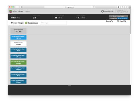
The layers are broken down on the left-hand side of the previous screenshot. We can see what action is being done at each level as the size that it adds to the overall image per layer.
