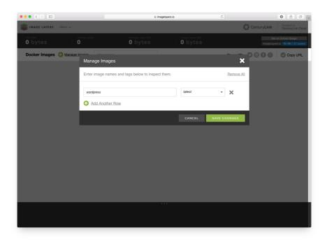
In this example, we are going to search for the *wordpress* image and select the **latest** tag. Now, you can search for any image and it does do autofill and then you can select any tag as well. This could be useful if you have, say, a staging tag and are thinking of pushing a new image to your latest tag, but you want to see what impact it has on the size of the image.
