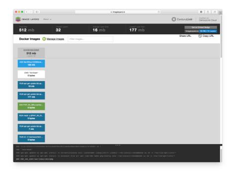
Upon hovering on a particular layer, you will be given information on it at the bottom of the screen in a black box. This will show how each action is layered one after the other so as to help see the command structure of the image.
