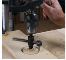
**Use it safely.** Use a circle cutter in the drill press only. Set the speed well under 500 rpm, clamp down the workpiece, and feed the cutter slowly for great results.
