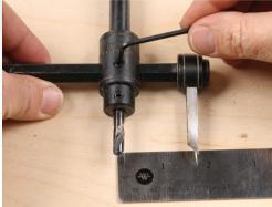
**Infinitely adjustable.** The swing arm can be adjusted for holes from 2" to 6" in diameter. Always lock the arm tightly.
