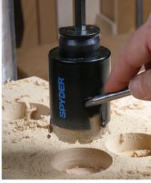
Pull the plug. After a holesaw cuts through the workpiece, you'll have to pry out the plug buried inside the bit.
