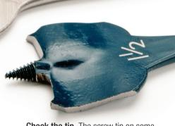
Check the tip. The screw tip on some spade bits can cause an aggressive feed rate. Don't use these bits in a drill press, and be wary of jamming.
