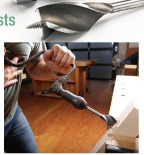
Hand power. Using an auger bit in a hand brace gives you more control than using a power drill.
