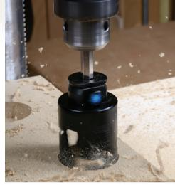
Fewer teeth, faster action. Holesaws with fewer teeth have long slots for clearing chips. which makes them work much better than holesaws with continuous teeth around the rim.
