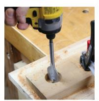
**Stopped holes, sort of.** A spade bit can drill a stopped hole, but the long center spur leaves a deep, narrow hole in the middle.
