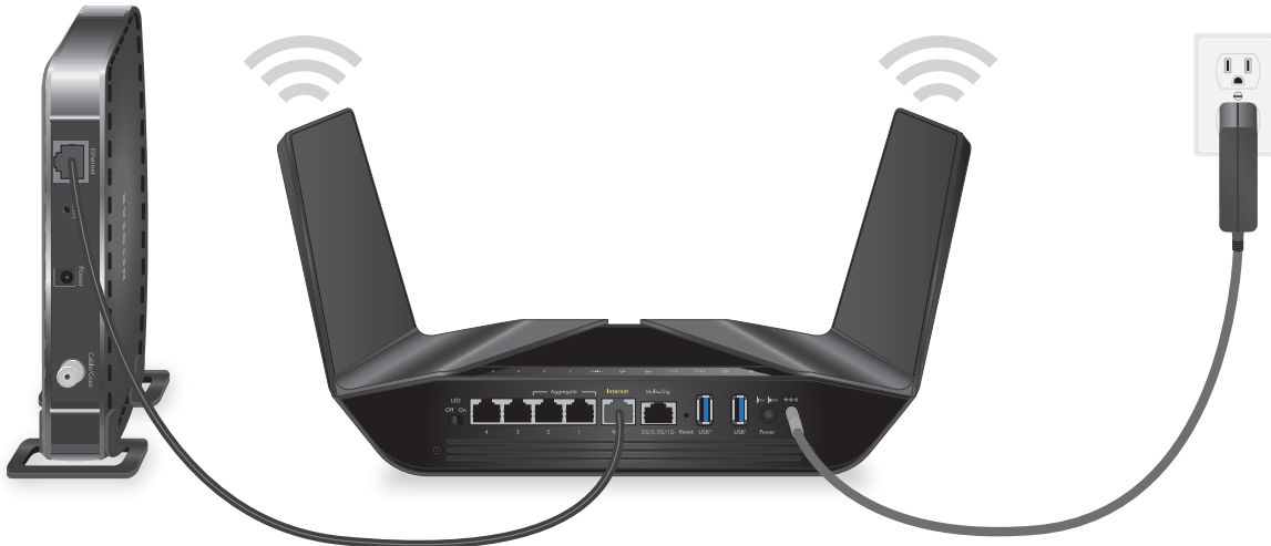
Figure 6. Cable your router
