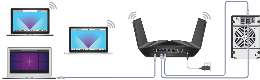
Figure 7. Ethernet port aggregation to a LAN device
